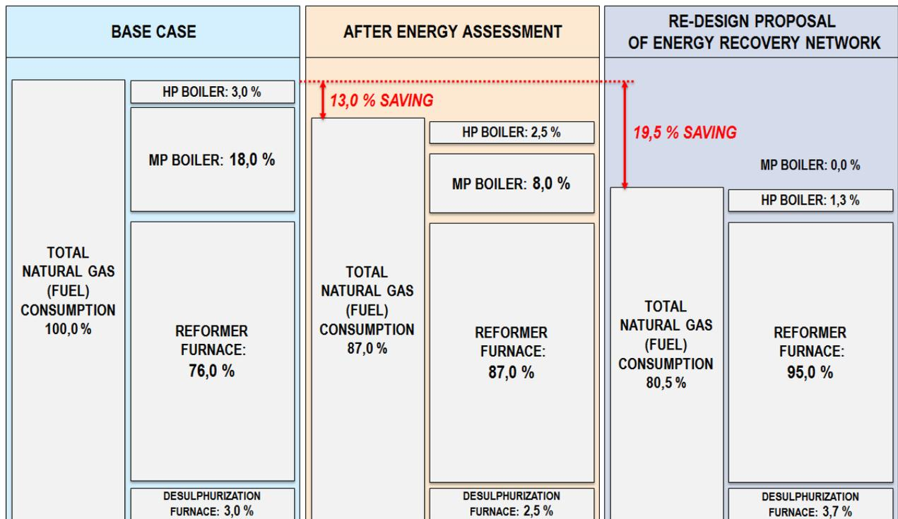
Figure 9 - Global potential for reduction of energy consumption of the site
