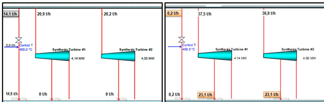
Figure 4 - Enabling extraction in syngas compressor driving turbine. Operation conditions in existing (above) and new situation
