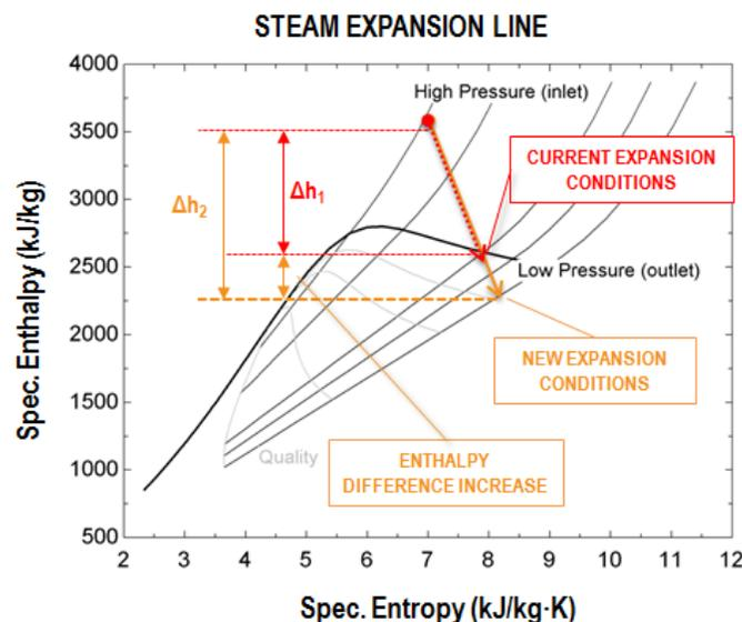
Figure 2 - Reducing condensing pressure in steam turbines. Schematic Mollier diagram
