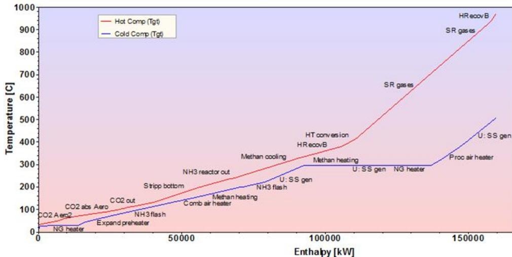
Figure 6 – Heating and cooling demand of the process. Thermal composite curves
