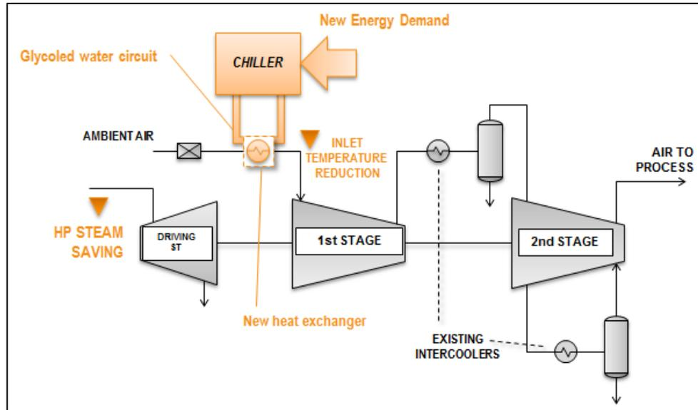
Figure 5 – Inlet and intermediate cooling in air compressor
