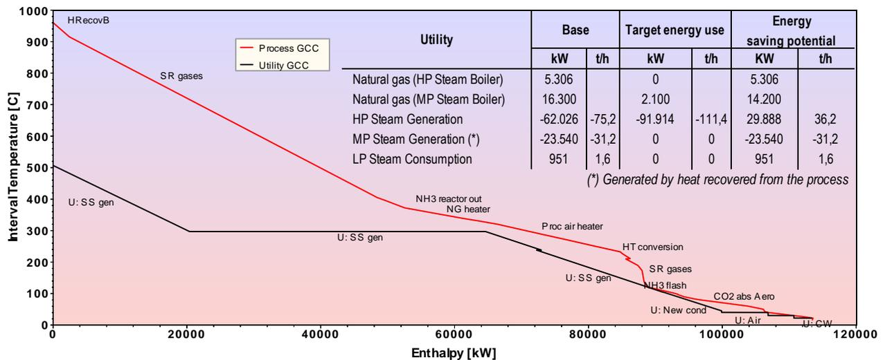
Figure 7 - Grand composite curve and potential energy savings
