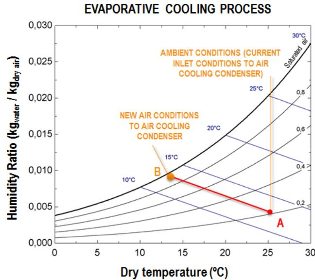
Figure 3 – Psychrometric diagram of an evaporative cooling
