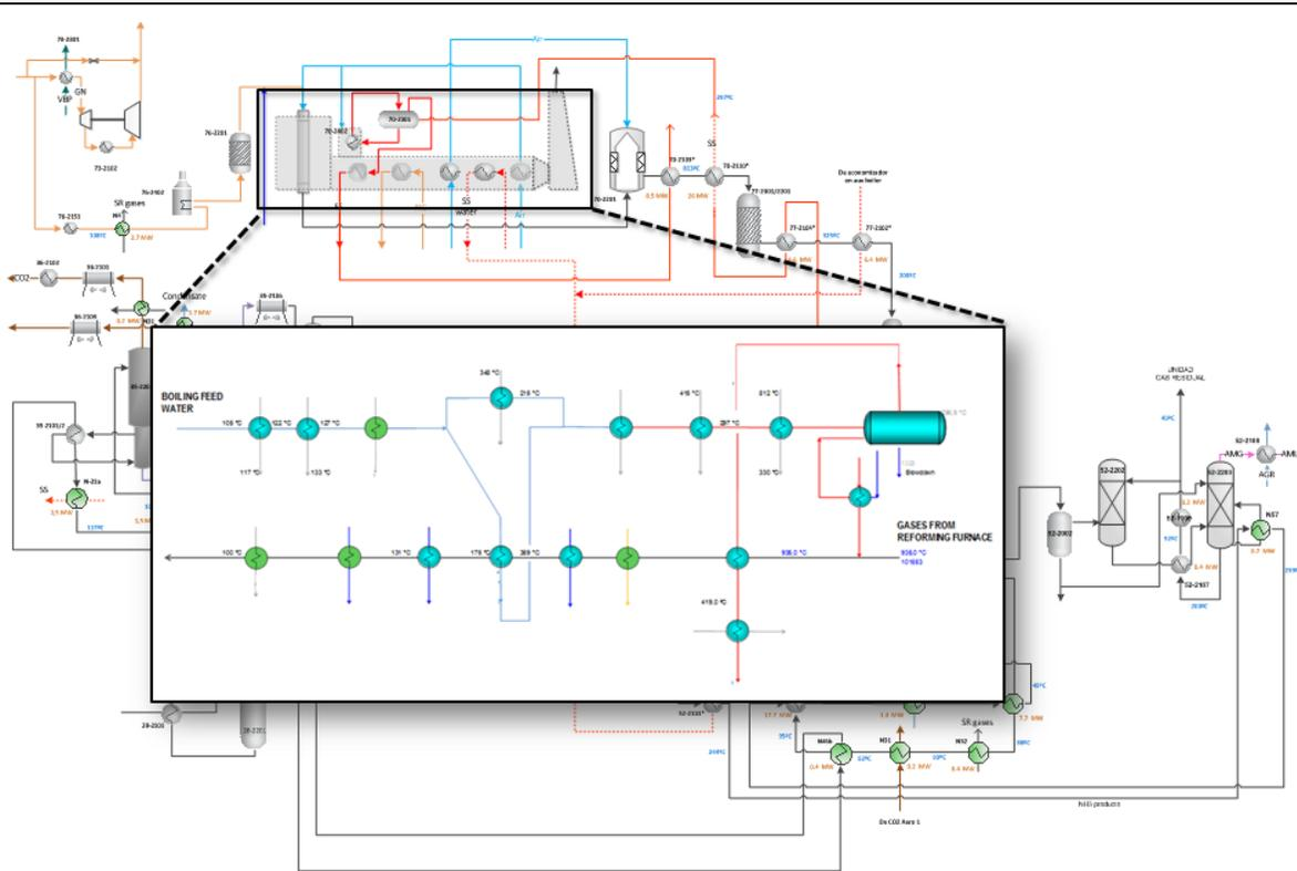
Figure 8 - Heat recovery exchanger re-design
